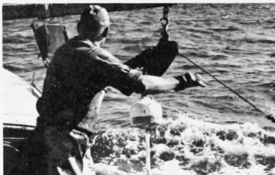
D. Placing rope over davit (note hydraulic pot hauler).
